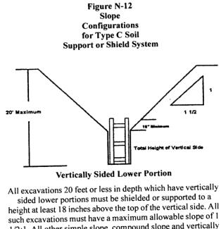
such excavations must have a maximum anowable slope of 1 1/2:1. All other simple slope, compound slope and vertically sided lower portion excavations must be in accordance with options permitted under RCW WAC 296-155-657(2).
