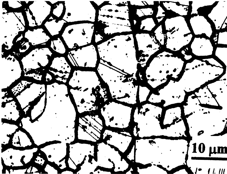
Figure 6 Heavily sensitized stainless steel microstructure. 4 (mag 2000x)
